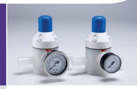
The pressure reducing valves V82 reduce pressure to a given value. They adjust themselves to the set working pressure and maintain it on the downstream side irrespective of fluctuations of inlet pressure or changes in flow demand.
