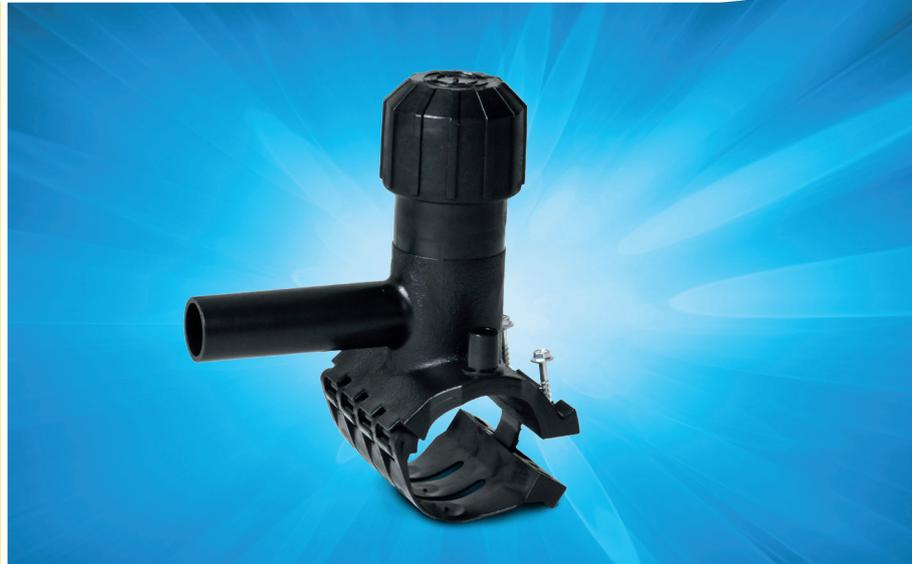
The AGRU tapping saddle creates branches on gas pipes under full pressure („hot tapping“) without interrupting the operation. This pressure tapping fitting is characterised by quick, easy and safe installation. Manufactured from stress crack-resistant PE 100-RC, the AGRU tapping saddle stands for maximum reliability during installation and subsequent operation.
