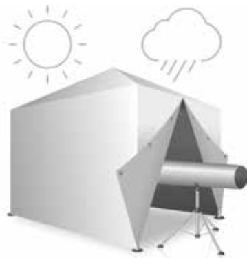
Figure C.1: Preparation of the welding zone acc. to DVS
