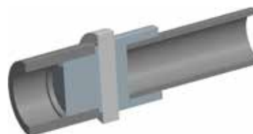
Figure C.8: Alignment and heating up
