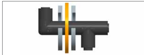
Figure A.20: Step 3: Heating the joining areas
