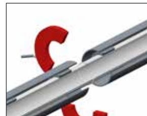
Figure A.16: Step 2: Heating of the outer pipe with a split heating element
