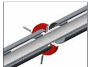
Figure A.16: Step 2: Heating of the outer pipe with a split heating element
