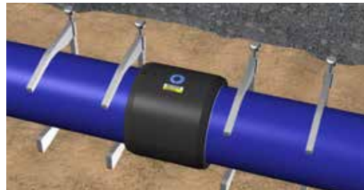
Figure D.20: Fixed welding components
