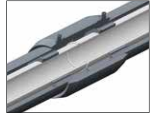
Figure A.13: Inner pipe welded with butt welding
