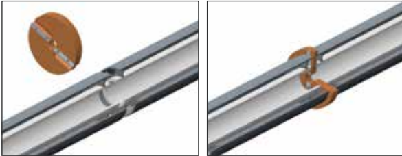
Figure A.8: Step 2: Planing of the joining areas
