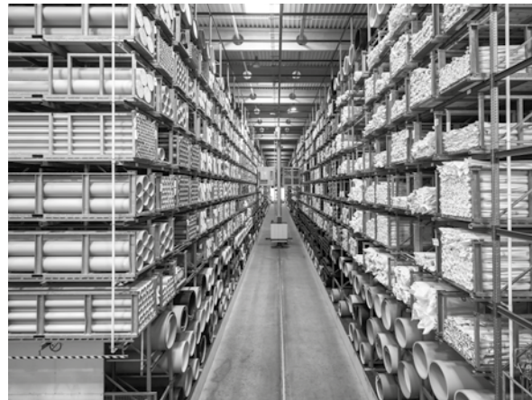
Figure B.2: Horizontal pipe storage
