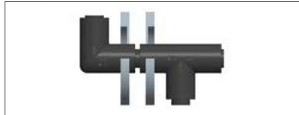
Figure A.18: Step 1: Control the offset on the inner pipe
